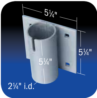
DE99014F Multi-Anchoring Leg Holder. Bolts to side of dock frame to anchor it in place yet allows vertical movement for water variances.
